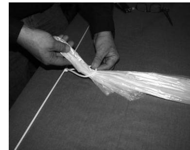
**Note:** the open end should never be used to attach the bag. It will catch air, inflate and will not go through the hold down pulleys and can get caught on corner pulleys.
